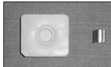
**Fig 1. Putty index and metal cylinder for fabrication of discs**
